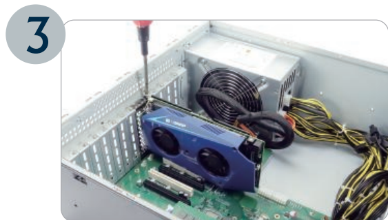
3 Press down to seat the Mustang-200 correctly in the slot. Install the bracket screw to secure the Mustang-200. 將Mustang-200完全插入機板PCI-E插槽後，鎖上擋板螺絲固定
