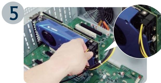
5 Connect the power cable to the power connector of the Mustang-200. 將電源線確實插入Mustang-200右上角電源接孔
